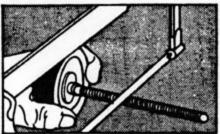
NOTE: Before screwing dial into the drive cam for the final time, lubricate the dial, dial ring and drive cam bearing surfaces. See "Helpful Hints" for proper lubricant.
