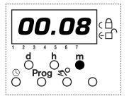
Press the "d" button until the current day of the month is displayed on the left side of the window. In this example, the TC-II has been set to the 30th day of the month.
