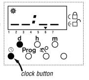
Hold down the "clock" button while pressing the "h" button until the current hour is displayed. The TC-II uses a 24 hour clock. In this example, the hour is 5 p.m., so the display should be advanced to 17 hours. A random number may appear in the minutes side of the window.
