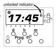
With the current time visible on the TC-II's display, press the "hand" button once. The locked/unlocked symbol will change from "unlocked" to "locked." When you close your safe, it cannot be opened until the TC-II reaches its next scheduled opening time.
