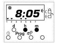
Press the "Prog" button until this display appears. The daylight savings time symbol may be different or absent, and the "locked/unlocked" symbol may show either state.
