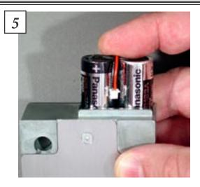
The battery pack will slide into the lock's battery compartment. Make sure the battery wires are routed up over the top of the pack, so the connector points directly toward the receptacle inside the lock case.
