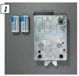
Your Pulsetronic lock requires two 3-volt lithium batteries. We recommend Duracell or Panasonic # CR123A cells. Always install NEW, unused batteries.
