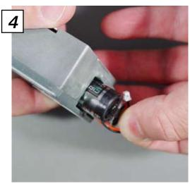
Here you can see the battery pack, wires, and white connector, as the battery pack is pulled from the lock case.
