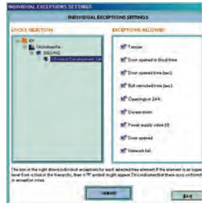
Establish operating parameters for the safe to help enforce security policy. Choose from a variety of common parameters such as door open time, bolt retraction time, network failure, power disruption and others.
