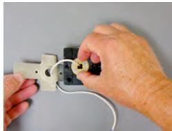
3. Remove and discard the plastic washer found under the cam plate. It is not used when locking bar extensions are added. Do not remove any of the lubricant you find under the cam plate.
