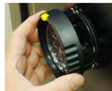
13. Place the keypad ring over the base and keypad. It should be slightly counterclockwise so that it will fit onto the base easily. After it is on the base, rotate it clockwise until it clicks into place. The yellow tab should be at 12 o'clock.
