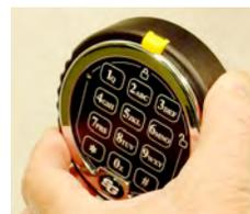
15. Push the keypad ring back against the base and turn it clockwise until it clicks into place. Test the lock function at least three times with the door open before closing the safe.
