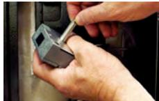
3. As you slide the last bit of cable through the spindle slot, place the cable into the lock body cam. The spindle and cam are configured to mate together.
