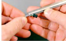
2. Insert the lock cable into the spindle slot as shown. Then slide the cable through the length of the slot.
