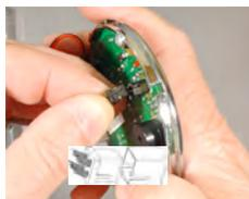
8. Plug the lock cable into the black receptacle on the back of the keypad. Note that there are two raised ridges on the cable plug and two matching slots in the keypad receptacle. Align these features before inserting the plug into the receptacle.
