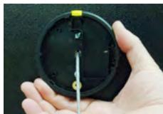
6. Pulling gently on the cable, move the keypad base against the safe door, and attach it using the two machine screws provided. Do not tighten beyond 15 inch-pounds (1,695 Nm).
