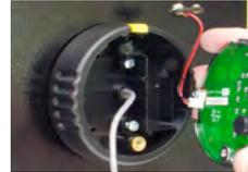
10. Place the battery cable through the slot at the base of the battery cable compartment and place the remainder of the cable in the compartment.
