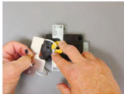
4. Place the extensions in the recessed channel provided. Seat the small extension tabs in the corresponding openings in the cam. With the extensions in place, return the cam plate to its original position. Fasten it in place with the two screws removed earlier.
