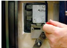
4. Place the end of the lock cable through the safe door from inside. Pulling gently on the cable insert the lock with attached spindle through the safe door so that it can be attached to the door's mounting plate with the three screws provided.
