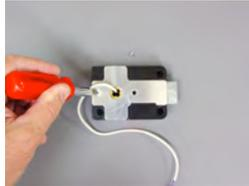
2. Remove the two screws that hold the cam plate to the lock body.
