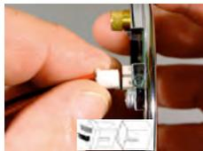
7. If not already attached, plug the battery connector cable into the white receptacle on the back of the keypad.
