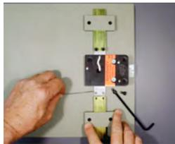
6. Here, vertical locking bolts are directly attached to the locking bar extensions. The attaching holes in the extensions will accommodate #8 or M4 screws. As the keypad is turned, the lock bolt and extensions will move toward the lock case, bringing the
