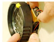
14. To install the battery, pull the yellow tab out slightly and turn the keypad ring counterclockwise. The ring will pull out from the base far enough to reveal the battery connector. Attach the battery and place it in the battery compartment.
