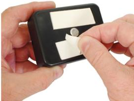
2. Select a good battery box location on the back of the safe door, inside the safe. Make sure the power wires from the lock body will reach it, and that the wires will not come into contact with moving parts. Use the included alcohol pad to clean the safe surface where the box is to be mounted, then peel the protective backing from the double-stick tape pads on the back of the battery box, and mount it to the safe. Press firmly into place.
