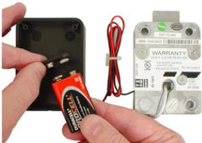
3. Run the power cable from the lock body to the battery box. Bundle and secure any excess cable using wire ties and tie blocks. Connect a 9-volt battery to the battery connector at the end of the cable.
