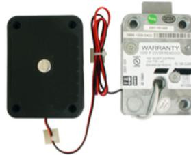
5. Place the cover on the box and secure with the screw you removed earlier. Be sure to secure the power cable near the battery box using a wire tie and tie block. Pull the tie tight so that it will act as a wire strain relief.
