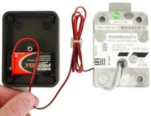
4. Place the battery inside the box. Make sure the power cable is in the slot at the end of the battery box before placing the cover on the box.
