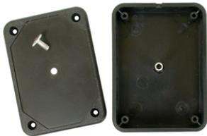
1. Remove the single screw in the center of the battery box cover and take the cover off of the box. Set the screw and the cover aside for now.
