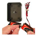
4. Inside the safe, bundle and secure any excess cable inside the safe using wire ties and tie blocks. Connect two 9-volt batteries to the battery connectors at the end of the cable.
