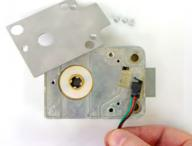
4. The switch comes with a very small piece of foam attached to the front, as shown here. The foam helps hold the switch in the lock cavity when the steel cover plate is attached.
