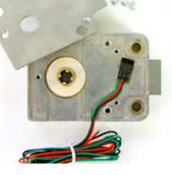
5. With the switch in place in the lock body cavity, route the three wires in the recessed channel. Make sure all three wires are completely within the channel so they will not be pinched or crushed when the steel plate is re-installed.
