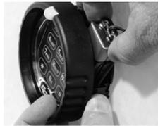
14. Push the keypad ring back against the base and turn it clockwise until it clicks into place. Test the lock function at least three times with the door open before closing the safe.
