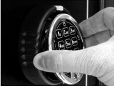
11. Keeping the lock cable and the battery cable in their respective compartments, place the keypad onto the base. The top seats into the base first, then the bottom.
