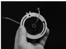
5. Place the lock cable through the center of the keypad base as shown.
