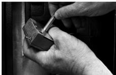
3. As you slide the last bit of cable through the spindle slot, place the spindle into the lock body cam. The spindle and cam are configured to mate together.
