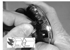
8. Plug the lock cable into the black receptacle on the back of the keypad. Note that there are two raised ridges on the cable plug and two matching slots in the keypad receptacle. Align these features before inserting the plug into the receptacle.
