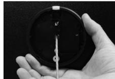
6. Pulling gently on the cable, move the keypad base against the safe door, and attach it using the two machine screws provided. Do not tighten beyond 15 inch-pounds (1,695 Nm).
