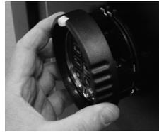
13. To install the battery, pull the keypad tab out slightly and turn the keypad ring counterclockwise. The ring will pull out from the base far enough to reveal the battery connector. Attach the battery and place it in the battery compartment.
