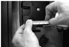
1. Measure the safe's door thickness (distance from the mounting surface for the lock to the mounting surface for the keypad. Add 3/4" (19 mm), and cut the aluminum spindle to this length.
