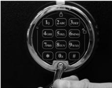
12. Install and tighten the keypad holding screw as shown. Use the one-way security screw for EN1300 applications. The Phillips screw is acceptable for all other applications. Once the screw is in place, cover it with the self-stick S&G logo after peeling the protective film off of the logo.
