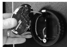
9. Place the lock cable into the recessed area of the keypad provided for it on the left side.
