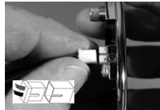
7. If not already attached, plug the battery connector cable into the white receptacle on the back of the keypad.
