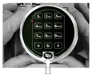
**Step 2**—Turn the keypad over and remove both batteries. This is best done by grasping the bottom of a battery and pulling it gently away from the keypad circuit board. Do not use any type of tool to pry a battery from its holder.
