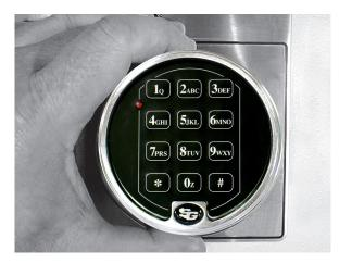
**Step 6**—Check the **master code** and all **user codes** at least three times *with the safe door open*. Close the safe door only after the lock has been thoroughly checked to make sure it's operating properly.
